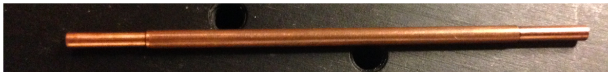
Figure 8 Copper electrode. Tips on either end are sharpened in order to cleanly break the burst-membrane. The double ended design allows a single electrode to be used twice before needing to be re-machined.
