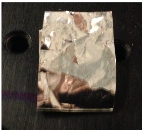
Figure 7 Foil used to protect the sample from contamination by pressurization fluid. Visible here is the folded piece of aluminum coated Mylar that wraps around a piece of foil.
