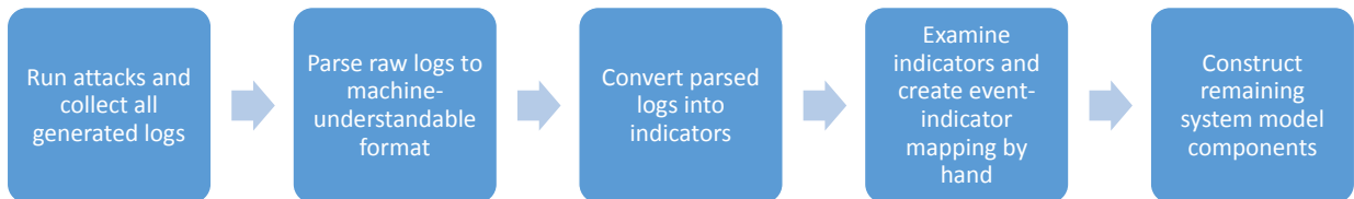
Figure 6.4: Flowchart describing the steps we take to generate the system model for the case study example given the system model and events defined in Section 6.1.
