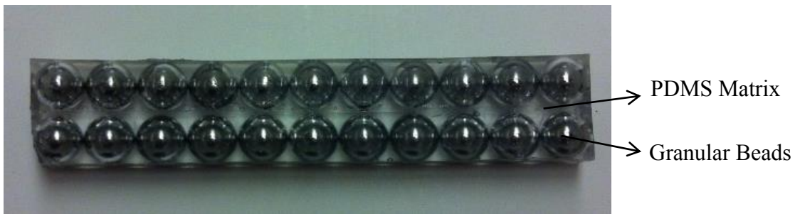
Fig. 5.1. Stainless steel granular chain embedded in PDMS matrix with a fixed later gap, 1.5 mm.
