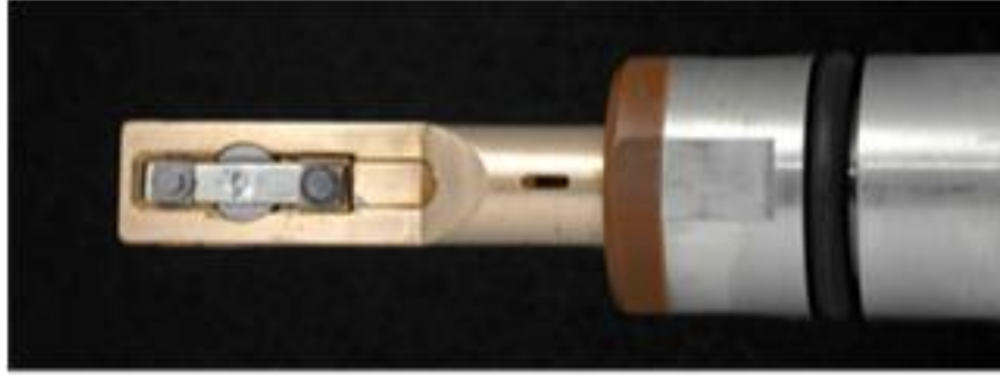
Figure 2.7: An in-situ TEM deformation holder with a sample loaded
