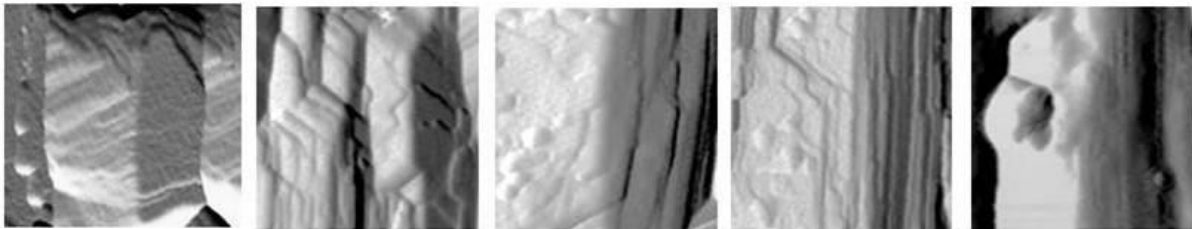
Figure 4.6: Square sections of AFM amplitude scans, 0.5\mu\text{m} \times 0.5\mu\text{m} , with facets of AIS(220) arranged such that details of both sides of a given facet are in view, and rotated so that corrugations run the same direction. The samples were grown at temperatures of, from left to right, 700^\circ\text{C} , 684^\circ\text{C} , 650^\circ\text{C} , 625^\circ\text{C} , and 584^\circ\text{C} .
