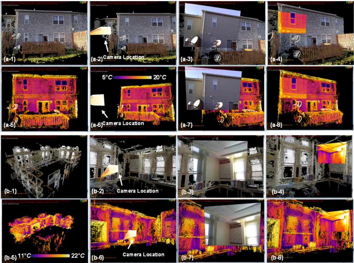
Figure 9.3 3D Building Geometrical and Thermal Point Cloud Models: (a) a Façade of the Residential Building (RB#1); (b) an Office Room of the Instructional Facility (IF#2)
