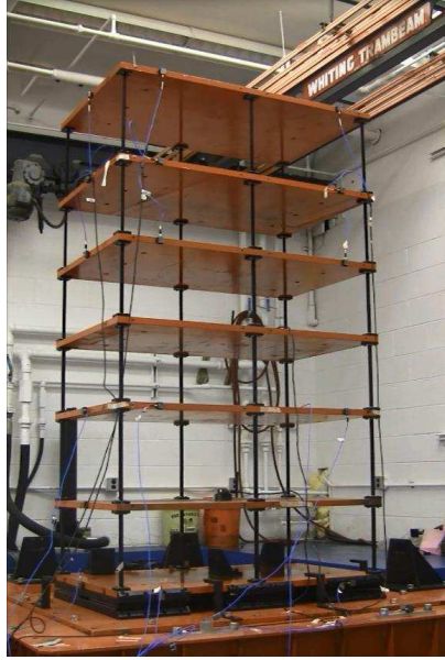
Figure 8.1: Photograph of the six-story base-isolated building model
