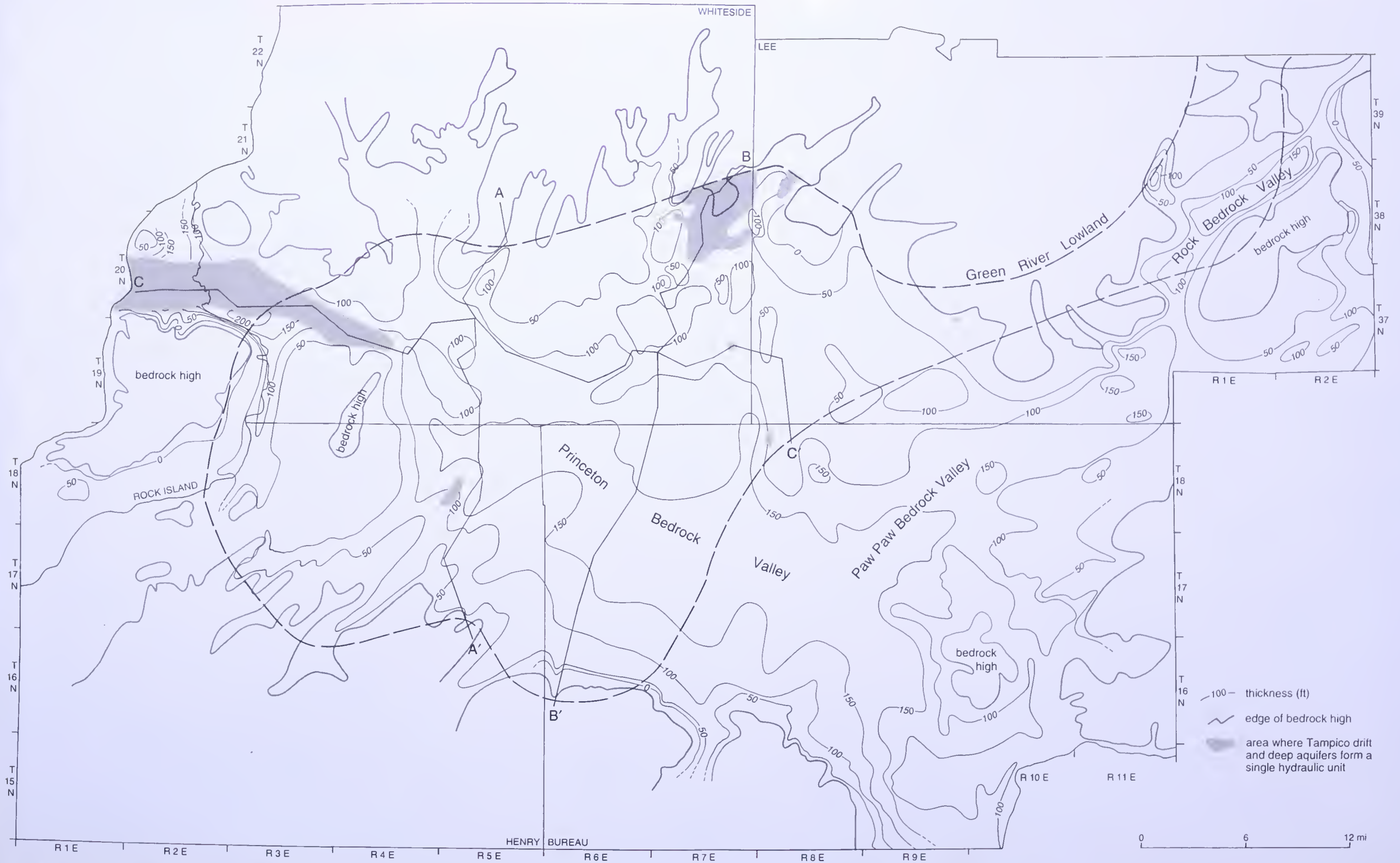
Plate 4 Thickness/estimated thickness of the bedrock valley aquifers, Green River Lowland area (lines of cross sections A-A', B-B', and C-C' are shown).
