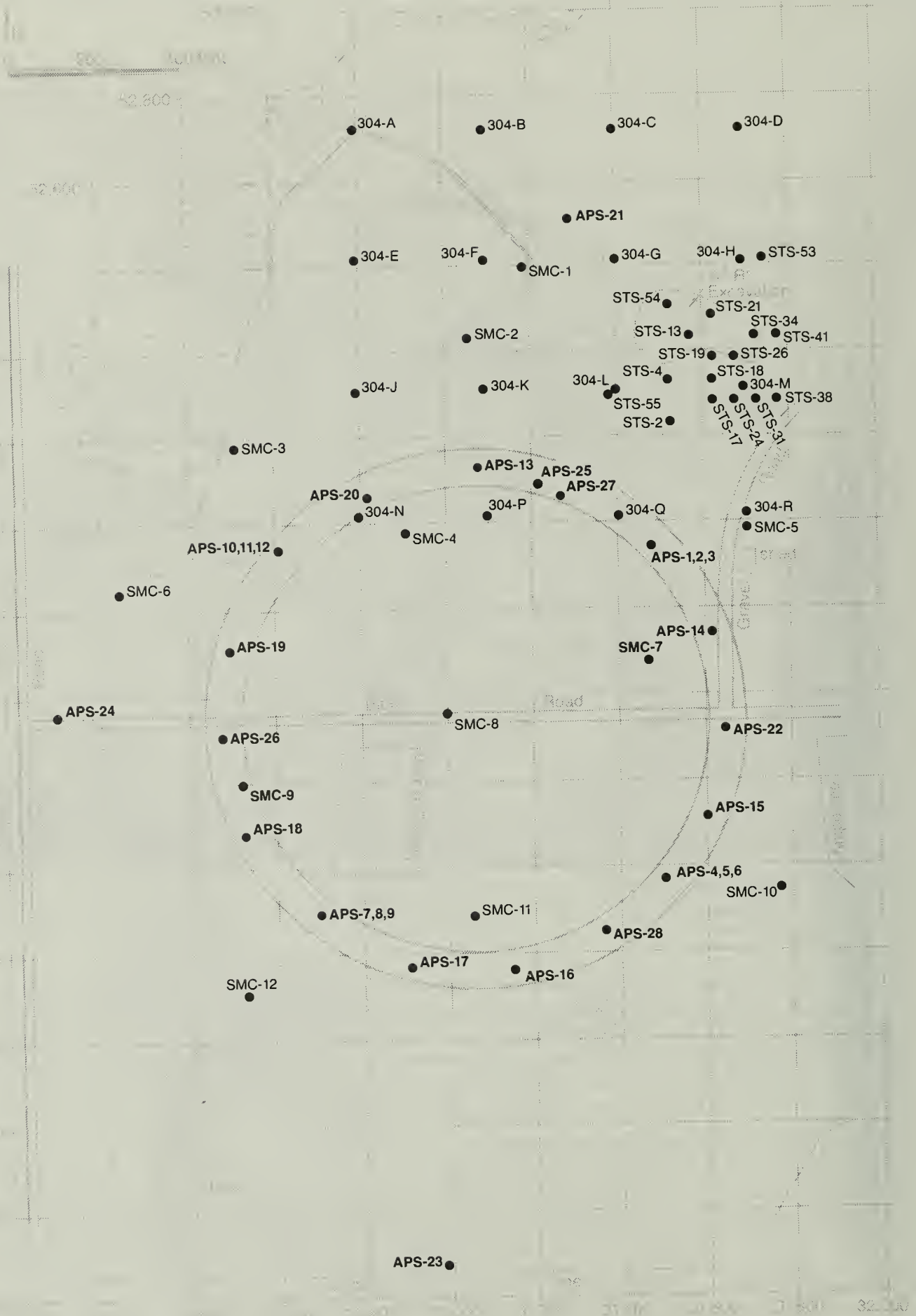
Figure 12 Location of all boreholes used to characterize the geology of the general APS site. Boreholes with APS prefixes were drilled specifically for this project.
