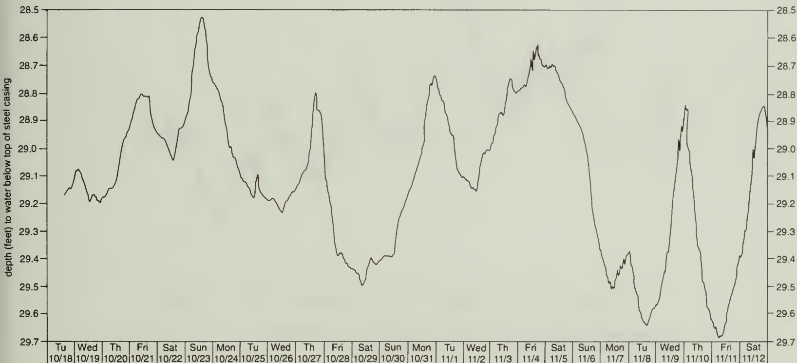
Figure 27 Hydrograph of the continuous water level recorder at APS-28 from October 18, 1988 to November 12, 1988. Head reduction and recovery of about 0.7 to 0.9 foot amplitude approximately twice a week are illustrated.
