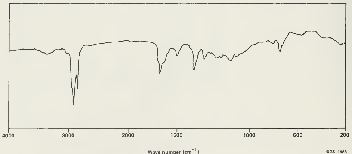
Figure 13. Infrared spectrum of the LC-4 fraction from the benzene extract of fly ash W1.
