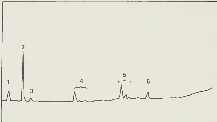
Figure 19. Gas chromatogram of the noncondensable hydrocarbons produced by pyrolysis at 450°C of fly ash 12. Peak identification: 1. methane; 2. ethylene; 3. ethane; 4. C 3 's; 5. C 4 's; 6. C 5 's.
