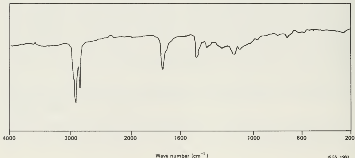
Figure 6. Infrared spectrum of the benzene-extractable organic material in fly ash I8.
