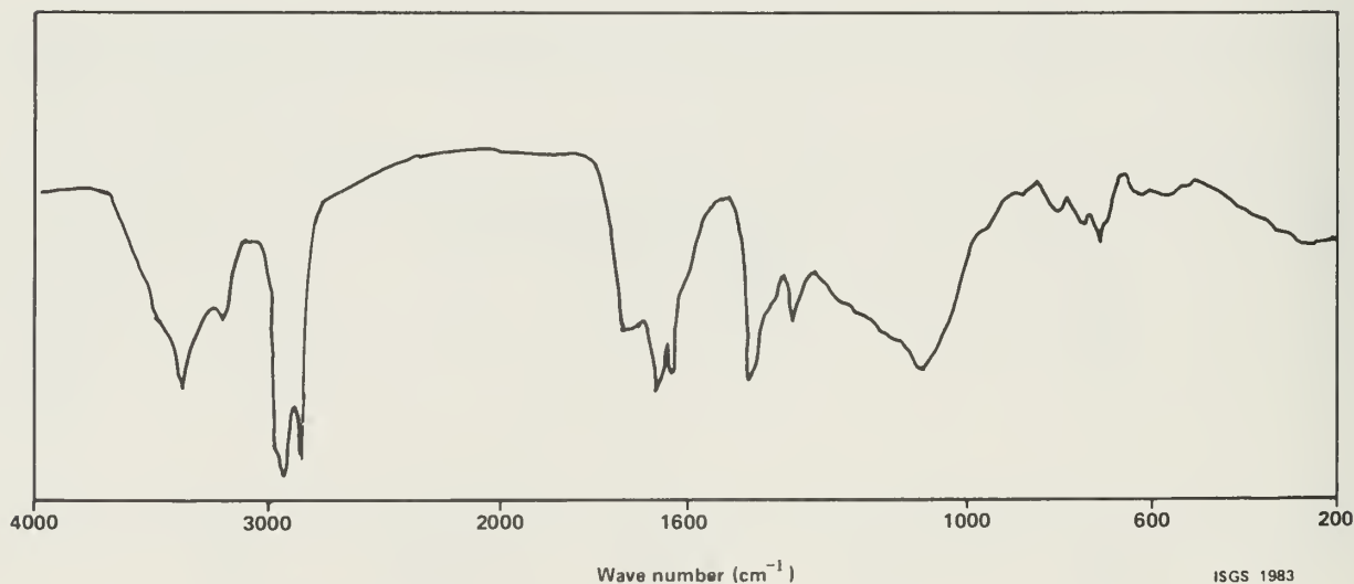
Figure 17. Infrared spectrum of the LC-6 fraction from the benzene extract of fly ash W1.
