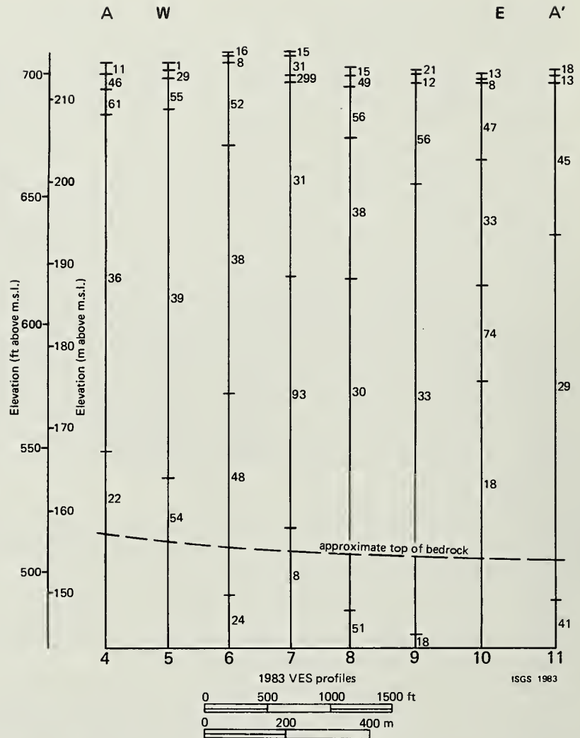
Figure 4a. Layering parameters ("true" resistivities and thicknesses) along line A-A', DeLand study area. "True" resistivity values are in ohm-meters.
