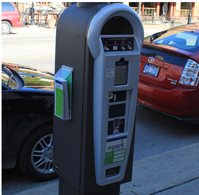
Figure 1.2. Fully-electric multi-space meter (Burdette, 2010)
