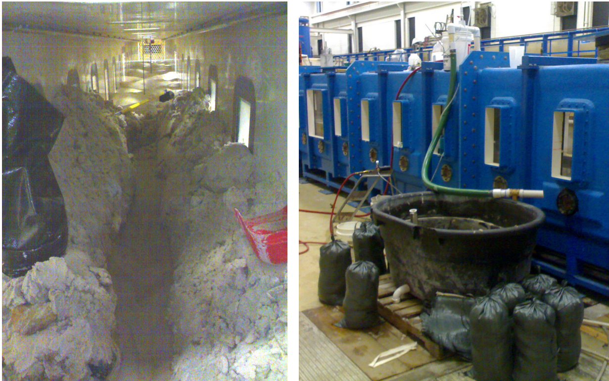
Figure 38. Pictures of the sand extraction process, by hand (left) and using a siphoning device (right).
