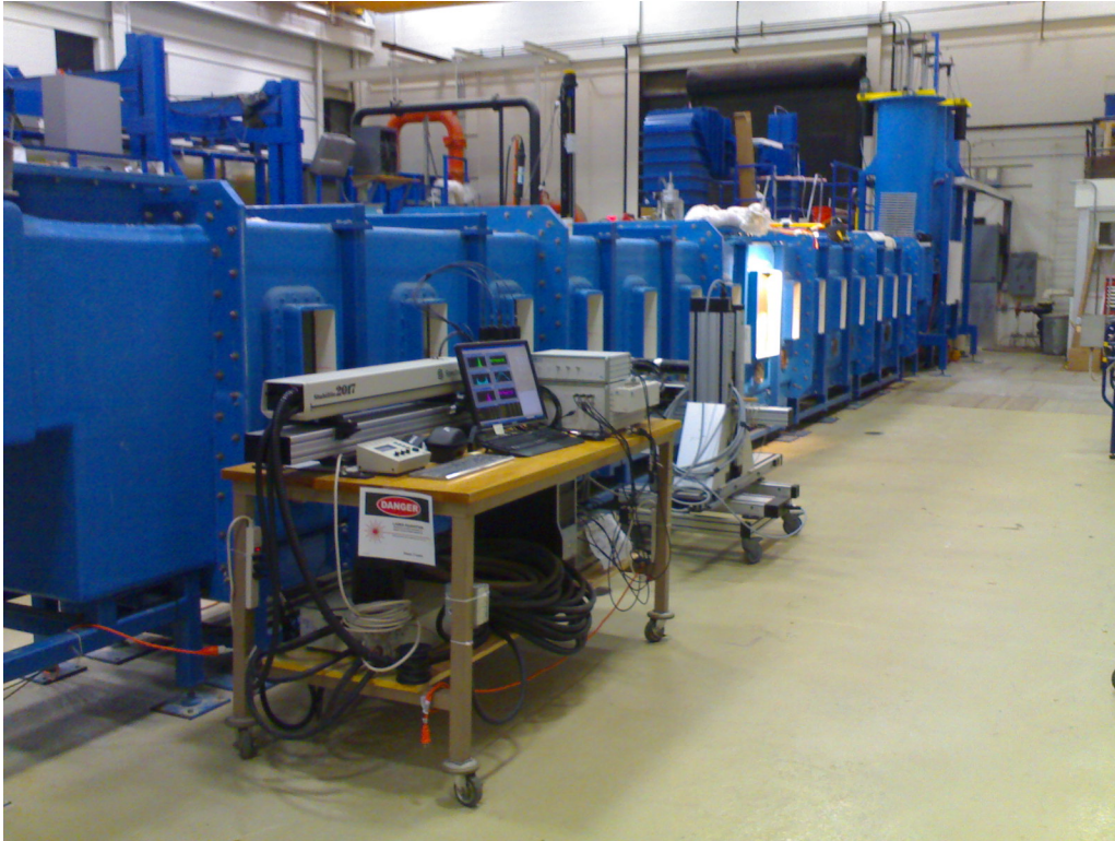
Figure 27. General view of the LOWST and the LDV system at the Ven Te Chow Hydrosystems Laboratory, UIUC.
