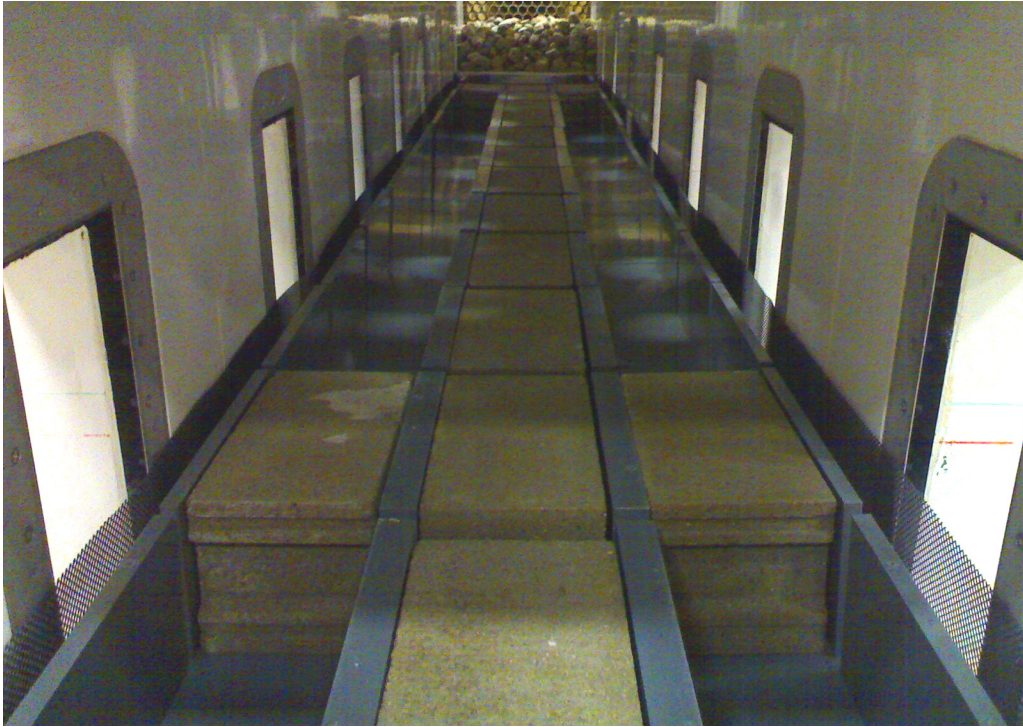
Figure 41. Picture of the inside of LOWST during assembly of the PVC bed. Concrete blocks were placed in between the vertical beams to add weight.
