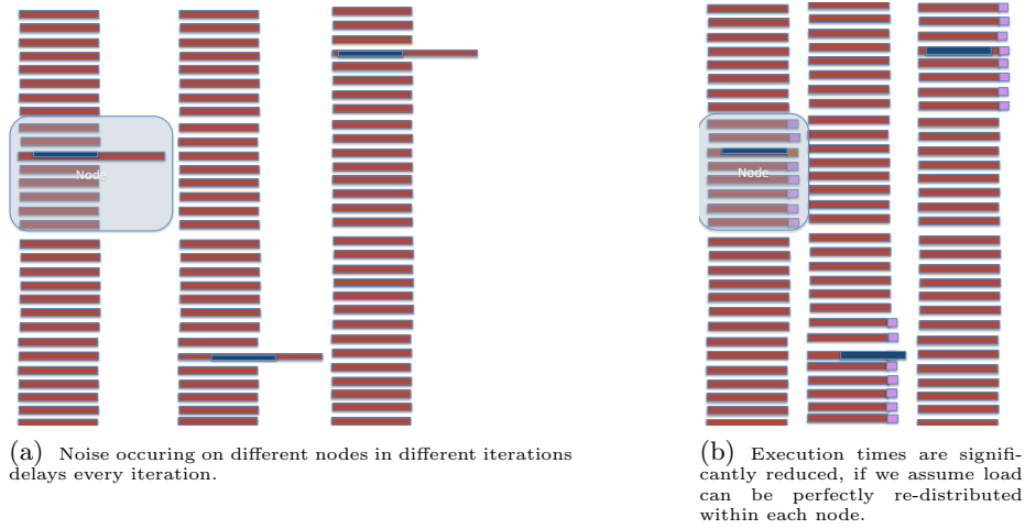
Figure 1.1: Schematics of application timelines showing how impact of noise can be mitigated by idealized within-node work re-distribution.
