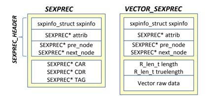
Figure 2.5: Internal representation of R objects.
