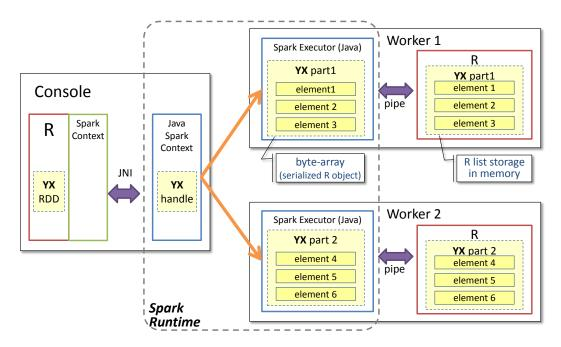
Figure 5.3: SparkR Architecture and Object Storage
