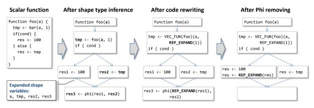
Figure 4.6: Function Vectorization Transformation Example
