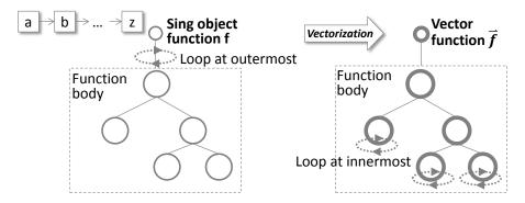
Figure 4.2: Function Vectorization Transformation
