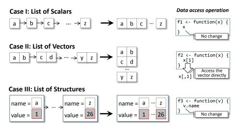
Figure 4.5: Data Access after PERM\_DOWN Transformation
