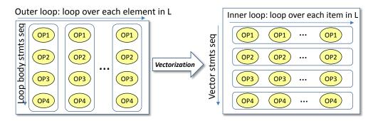
Figure 4.3: Loop Distribution in Vectorization Transformation
