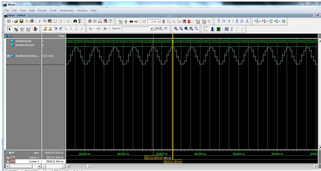
Figure 6.5: 32-bit 5MHz Traditional Spurs Gate-Level Simulation
