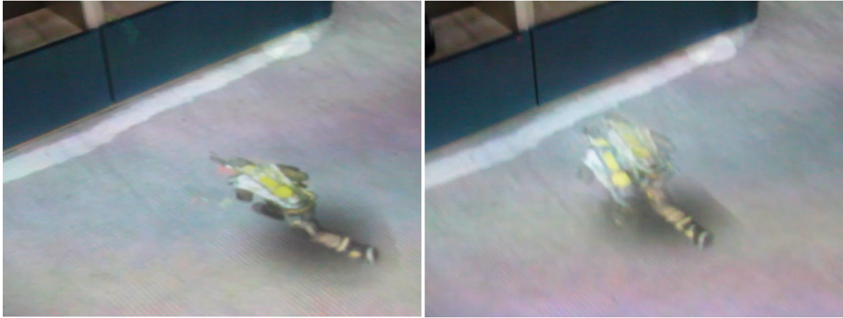
Figure 3.27: Calibration errors between units result in ghosting artifacts in projector overlapping regions. (left) The character in a single projector, and (right) in an overlapping region.
