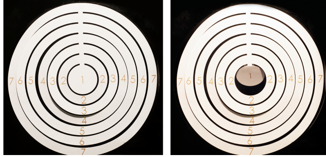
Figure 5.4: A paper target was used to measure accuracy performance. We show the target at its resting and hit state.
