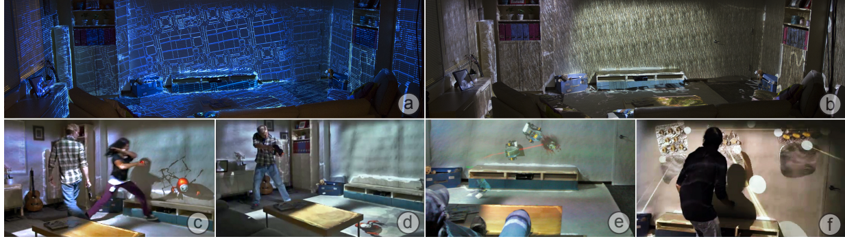
Figure 3.18: RoomAlive is a proof-of-concept system using multiple projector-depth camera units to transform any room into an immersive, augmented, magical gaming experience. RoomAlive captures a 3D scan of the room and adapts the gaming content to stuff in the room. It can transform a room into any environment imaginable including: (a) a Tron inspired game room, or (b) a swampy river. Users can play Whack-A-Mole and physically (c) whack or (d) shoot moles popping out of their floor, walls and couch. (e) Users can control a character running around their room and shooting enemy robots, by using a video game controller. (f) Users can play an adventure game in their living room, avoiding deadly blow dart traps with physical body movement. (All of the images in this paper were captured live; showing the real-time working prototype ).
