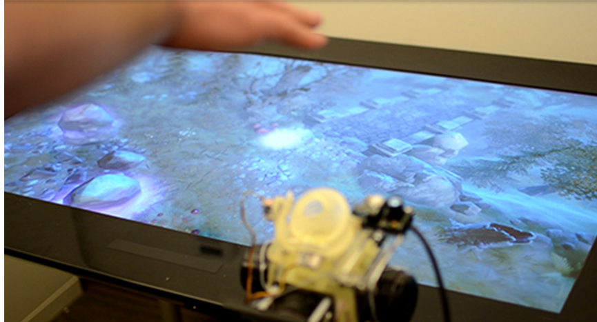
Figure 5.12: The user can feel textures of the virtual terrain.
