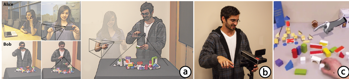
Figure 4.1: The (a) BeThere concept - a self contained mobile smartphone with integrated depth sensors. Bob is in need of help constructing a wooden block model and decides to capture and share a 3D representation of his local environment with remote user Alice. With Alice’s mobile device, she can perform spatial and gestural interactions that can be seen by Bob. In (b), a user is shown holding our proof of concept system that simulates a mobile smartphone of the future and (c) shows what a user like Bob sees in their mobile device. Here, remote user Alice is controlling a 3D virtual hand in a shared representation of the environment in order to show where local user Bob should place the physical blocks.
