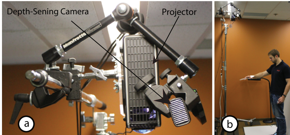
Figure 3.11: (a) LightGuide uses a single projector and depth sensing camera, (b) the projector and depth camera are fixed over the users body. .
