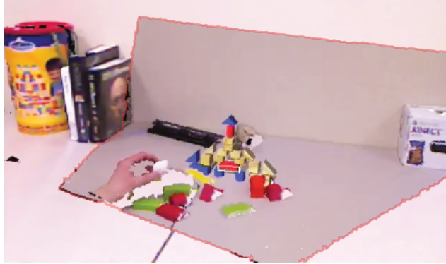
Figure 4.4: If remote user Alice is pointing at an object while Bob is looking away, then Bob has missed the interaction. Here, a user turns on a visual aid to see what the other user currently sees. This aid allows a user to ensure that an interaction (e.g., pointing) is seen by the other user.
