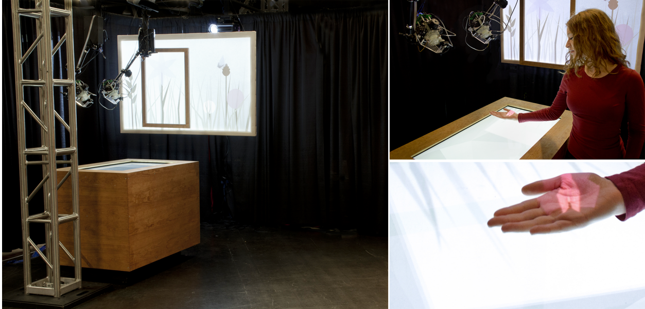
Figure 6.4: Free air haptics can be expanded into the real world with projected virtual imagery on physical objects.
