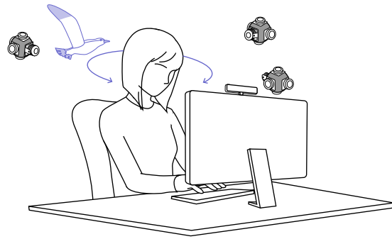
Figure 5.11: Continuous free air tactile sensations around the user. The user who is playing a game can feel virtual seagulls fly continuously around him.
