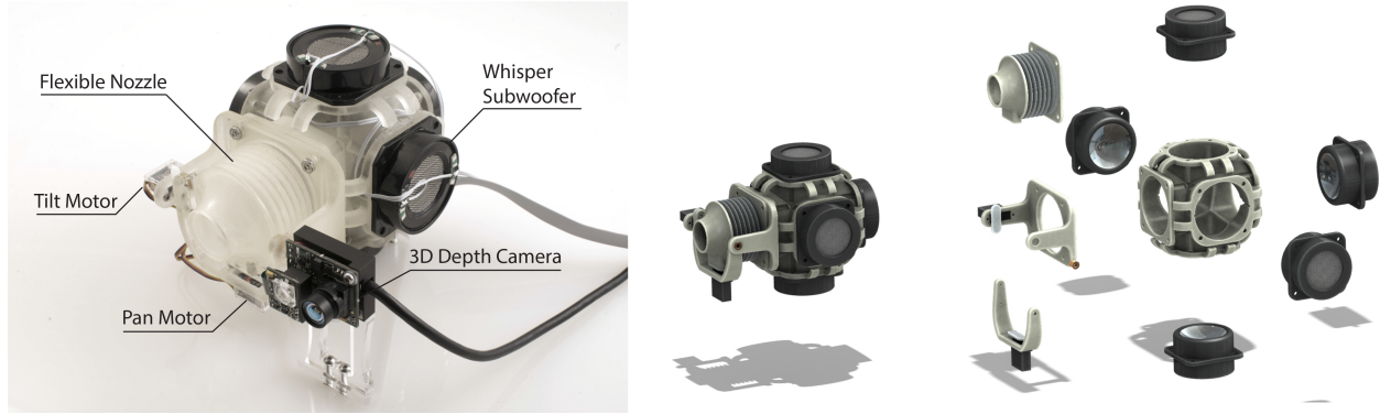
Figure 5.2: Top: a fully assembled AIREAL device. Bottom: an exploded view showing speakers, the pan and tilt motors as well as the 3D print-ed enclosure, flexible nozzle and gimbal structures.
