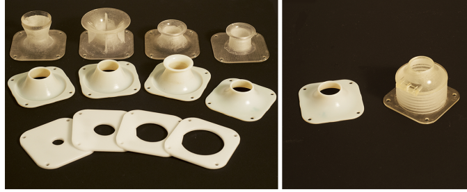
Figure 5.6: The various nozzle shapes and apertures tested and the final nozzle selection and its flexible equivalent.
