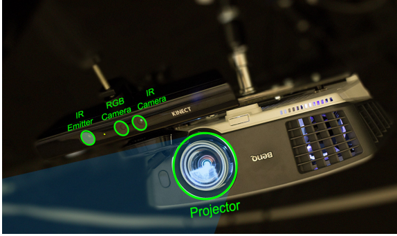
Figure 4.2: Each procam unit consists of a commodity wide field-of-view projector, depth camera and computer.
