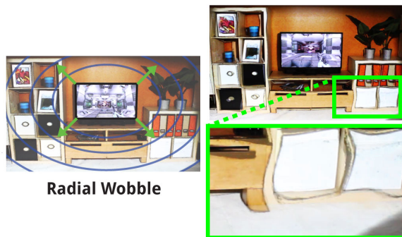
Figure 3.6: Radial Wobble : To create a ‘force field’ ripple effect, the physical surface texture is displaced with a radial expanding sinusoidal pattern.
