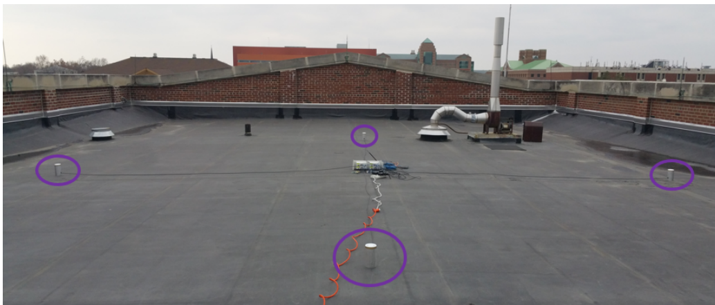
Figure 4.5: The antennas are placed at an approximately 10 m radius.
