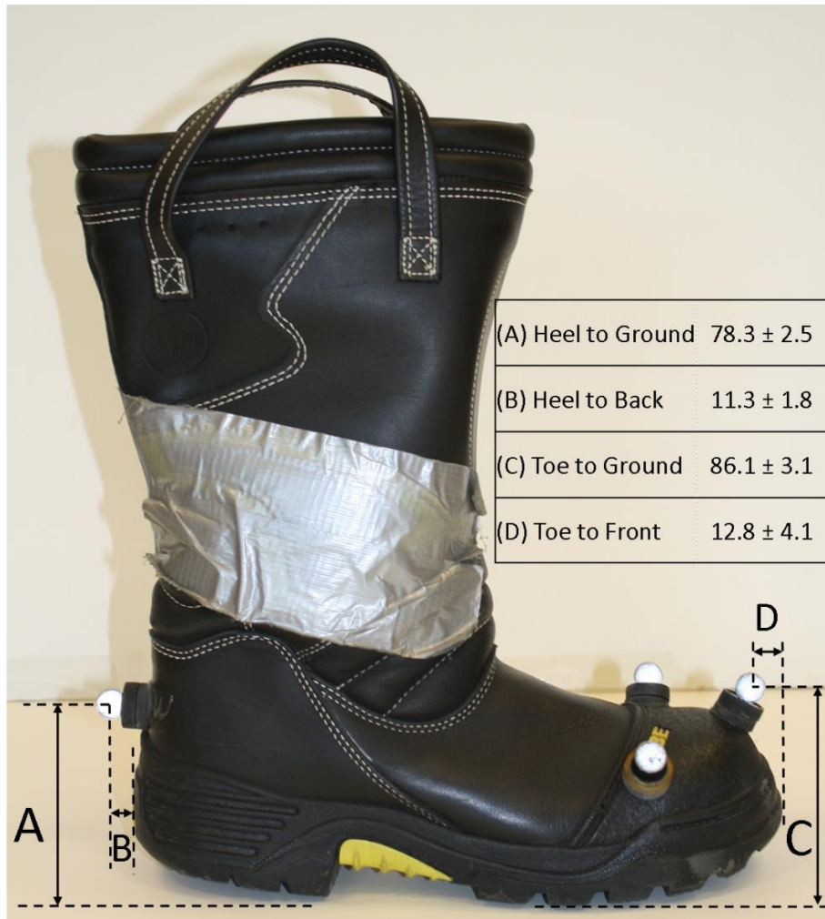
Figure 3. Boot marker setup. For reference only, offset distances between marker centers and relevant surfaces are identified as A-D. Table lists average ( \pm standard deviation) offset distances in mm over six boot sizes. Reflective areas on boots were covered to prevent cameras from falsely identifying them as markers.
