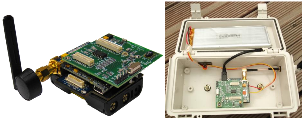
Figure 6.3. (a) Stacked WSS board with battery board and SHM-A sensor board, (b) enclosure for campaign monitoring applications (ISHMP 2014).
