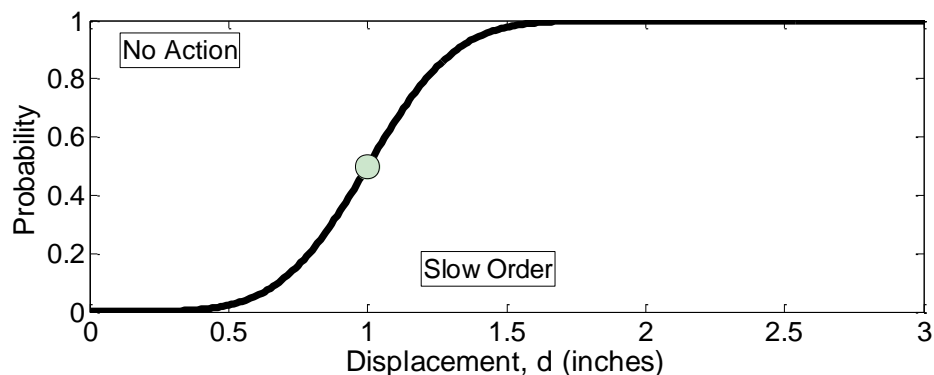
Figure 4.6. Fragility curve of bridge condition based on measured displacement under trains.
