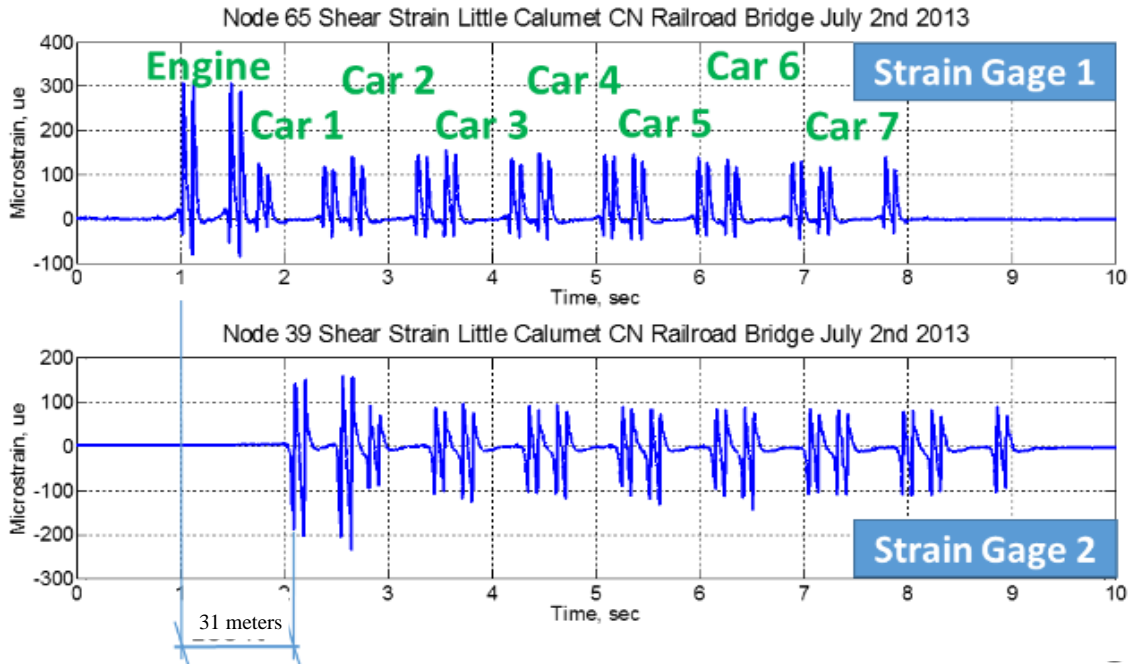
Figure 8.6 Estimation of train speed using two wireless strain gages installed in the rail.
