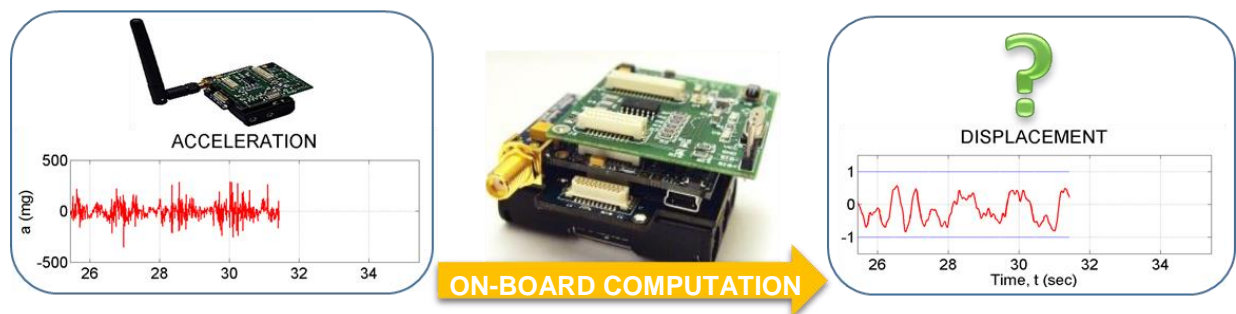
Figure 6.1. Reference-free displacement estimation using wireless smart sensors (WSS)
