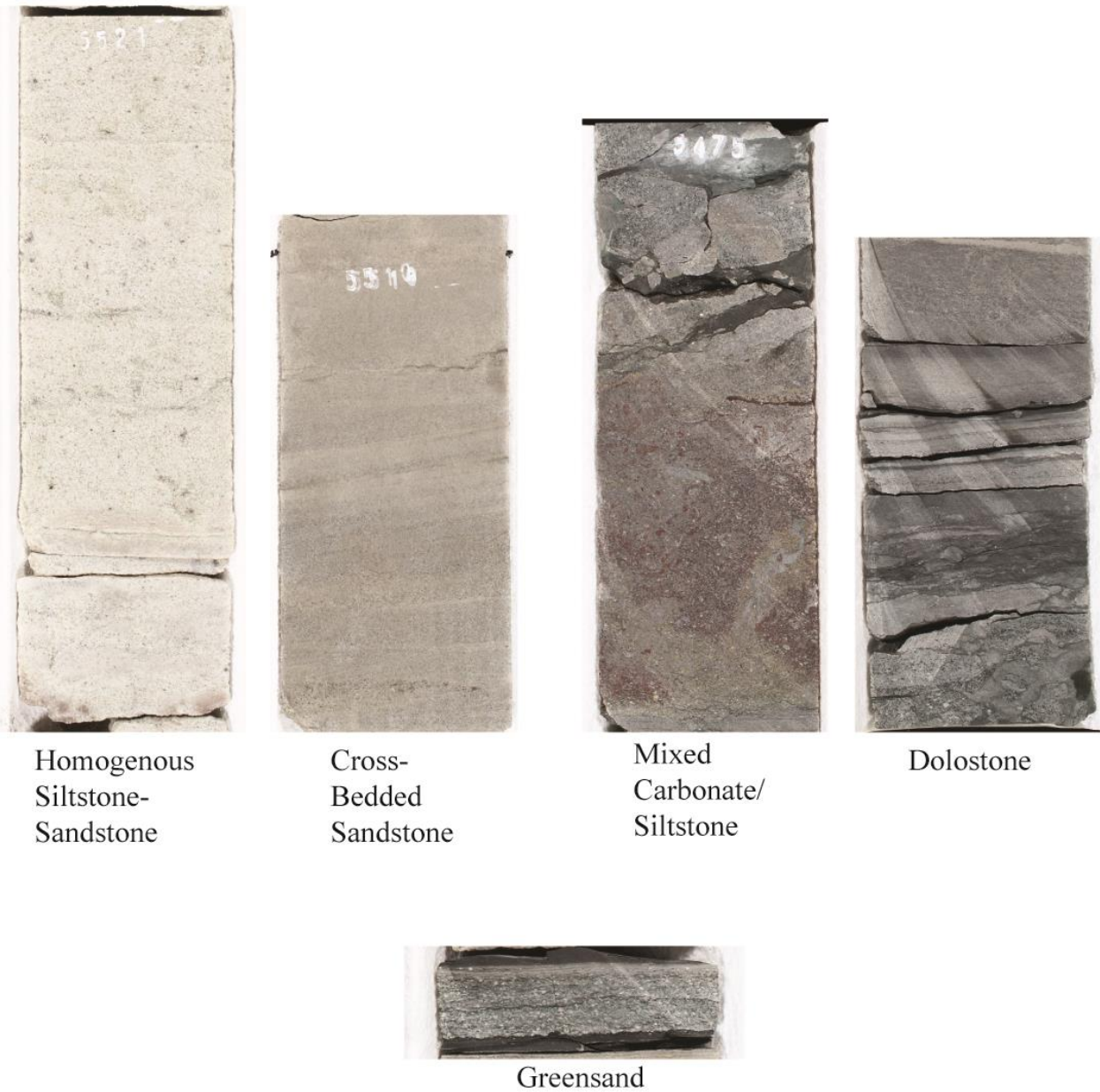
Fig A.2. Lithofacies found in the Eau Claire drill core from the VW#1 well (Units A-C).
