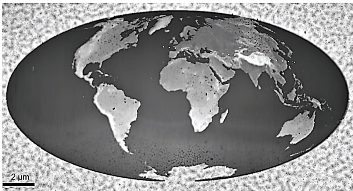
Figure 1.1 | AFM topographic image of a 3D world map written into a poly(phthalaldehyde) layer by thermally induced depolymerization via probe-based nanolithography (Reproduced with permission from Reference 16f. Copyright 2010 John Wiley and Sons).
