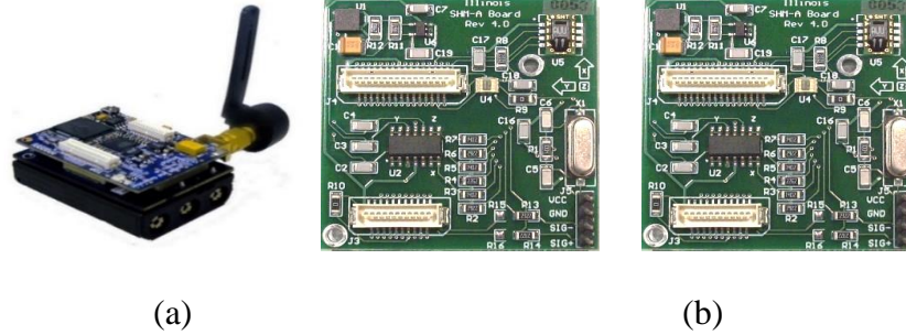
Figure 6.2. (a) Imote2 sensor board with antenna and stacked on battery board, (b) SHM-A sensor board (above and below views) (ISHMP 2014).
