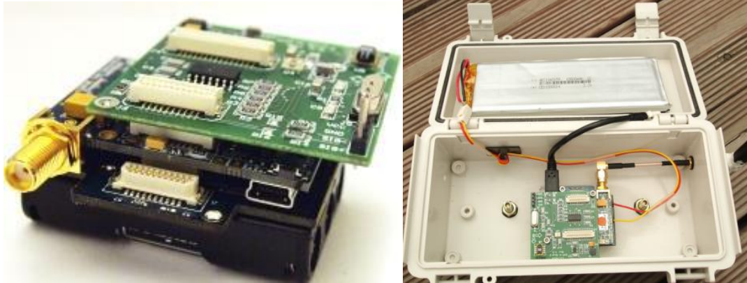
Figure 2.15 (a) ISM400 board stacked on Imote2, and (b) sensor enclosure assembly.
