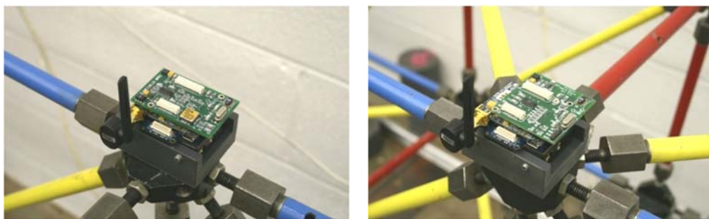
Figure 0.53. Imote2 sensor with SHM-H board (left) and with SHM-A board (right).
