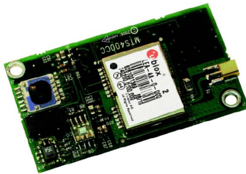
Figure 0.9. MTS420CC (with GPS module) for Micaz platform (MEMSIC 2011).
