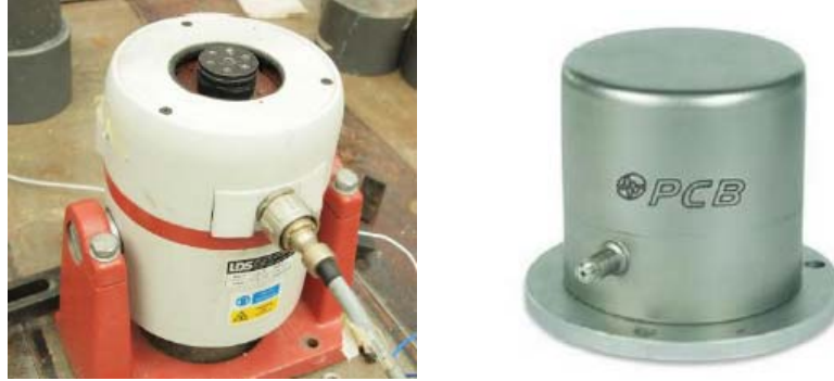
Figure 0.22. Electrodynamic shaker (left) and PCB393C accelerometer (right).
