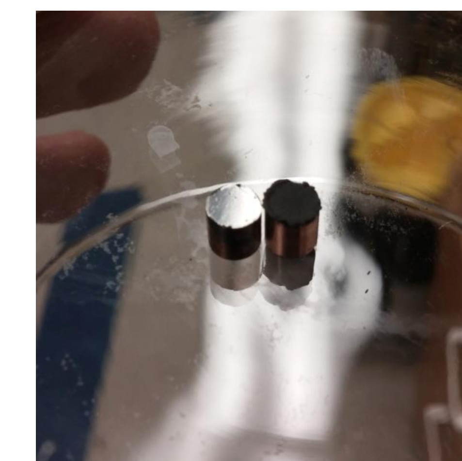
Left: polished graphite electrode Right: dried slurry (pre-polish)
