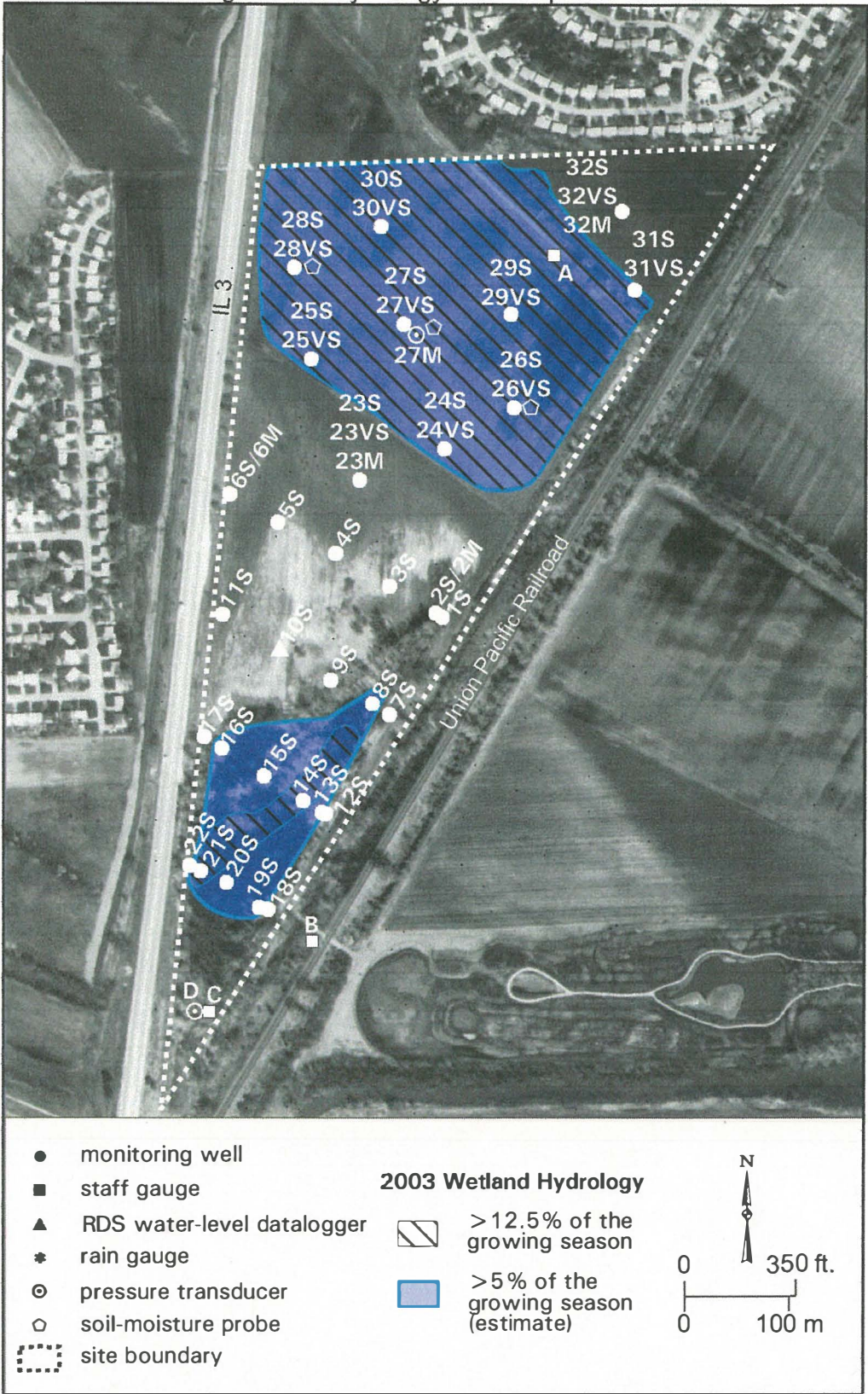
Areas exhibiting wetland hydrology in 2003 (map based on Illinois State Geological Survey 2001b, 2001c, 2003).
