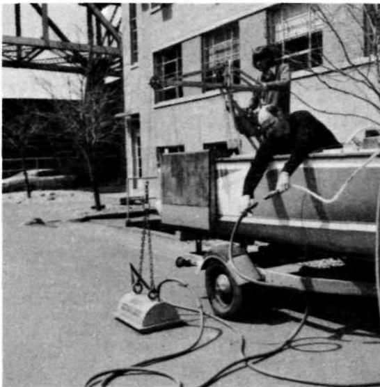
Figure 3. Discharge SOD sampler showing hose connections at pump (left) and probe installation in sampler (right)
