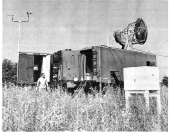
Figure 12. Buncombe radar site with wind set tower and cloud camera shelter (foreground)
