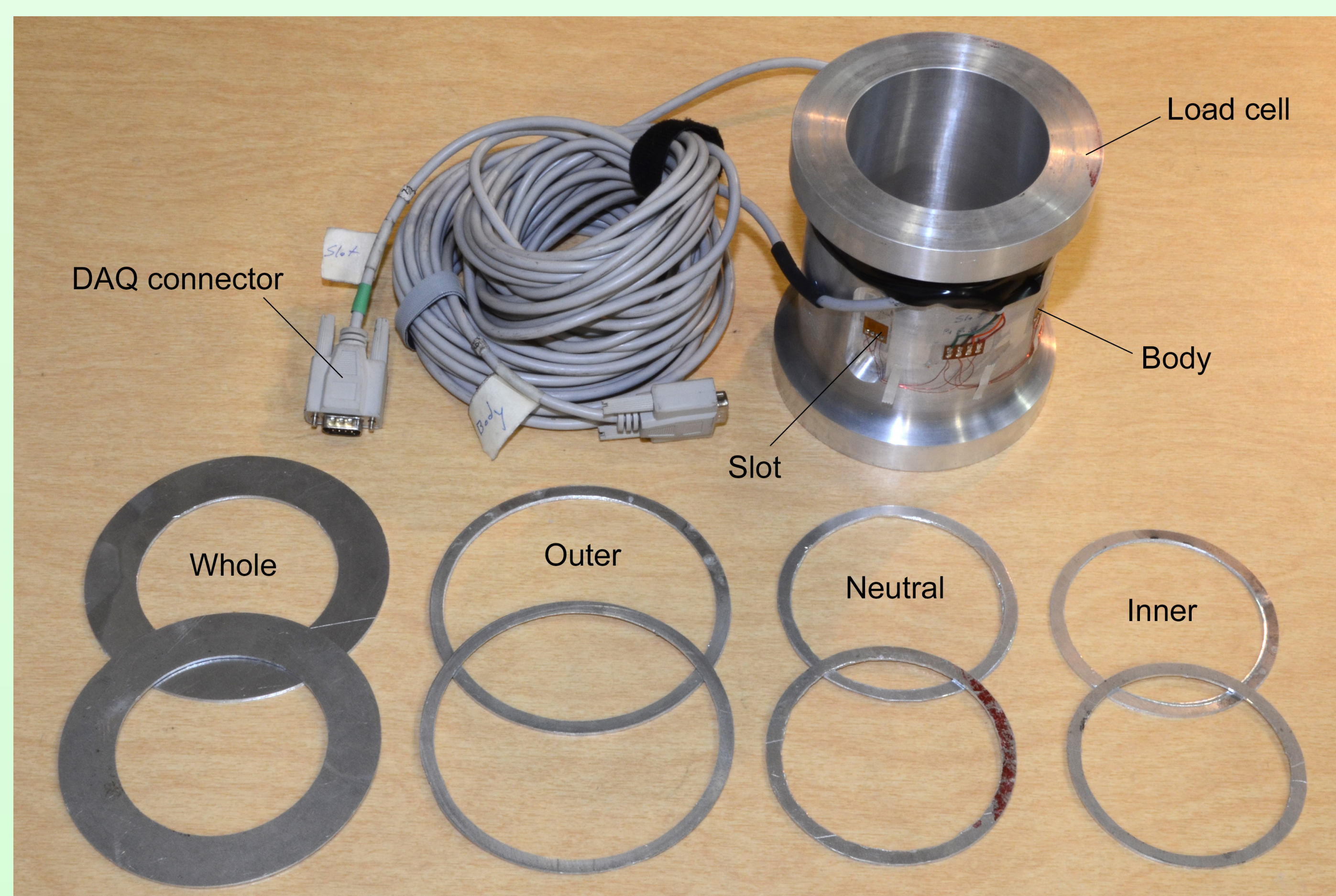
Figure 3: Load cell and metal rings. (Photograph courtesy of Prof. James W. Phillips.)
