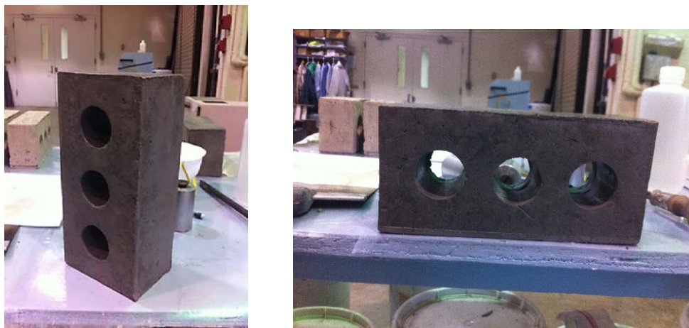
Figure 3: Brick unit after being removed from the mold.
