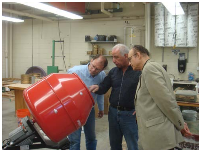
Figure 5: Drum mixer used for biomass concrete.
