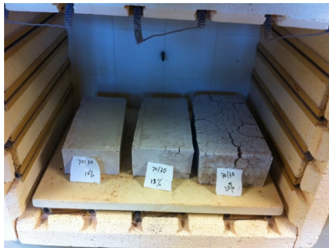
Figure 12: Surface cracking and expansion in bricks after firing (10%, 15%, and 20% ash from left to right).
