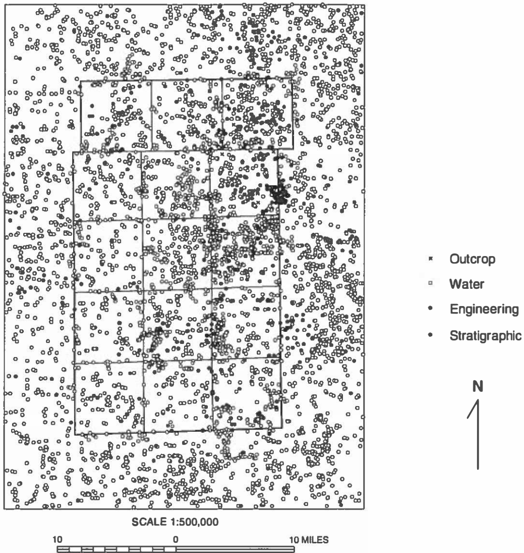
Figure 6 Distribution of primary wells in the study area used to generate lithostratigraphic surfaces.
