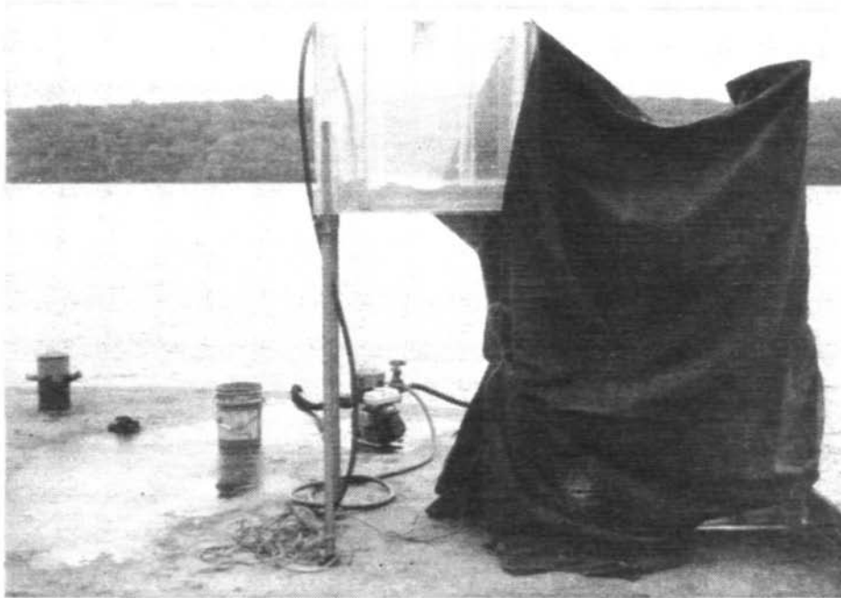
Figure 12. Closeup of weir box in the field, using tarp as a windbreak
