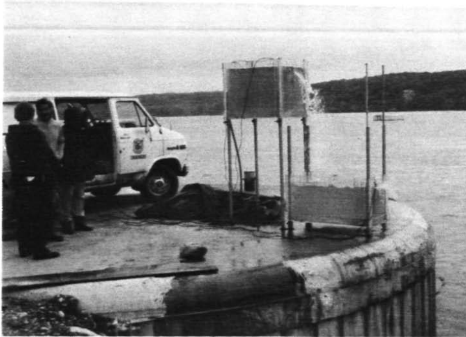
Figure 10. Weir box run in the field at the Starved Rock dam
