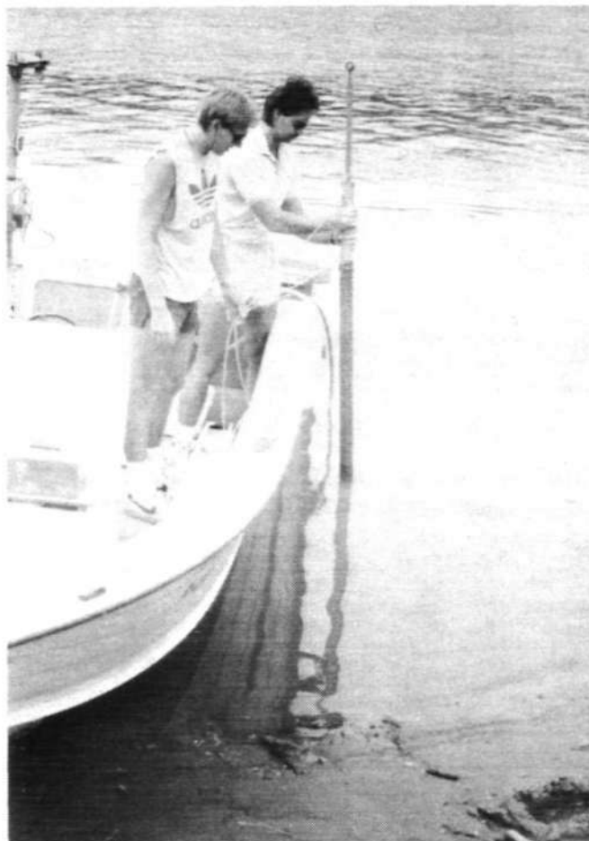
Figure 9. Sediment core sampling attempt near shore at Market Street outfall area
