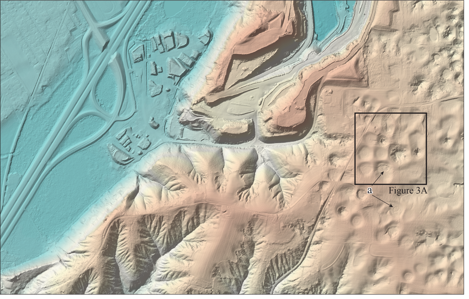
Figure 2A LIDAR digital terrain model (DTM) showing an area of about 1 1/2 square miles in western St. Clair County (T10N, R10W). A DTM represents only the ground surface, and is extracted from airborne LIDAR data using automated filtering methods to produce what is commonly referred to as a "bare-earth" point cloud. St. Clair County is part of the Illinois Sinkhole Plain, which contains the highest concentration of karst features within the state. It is estimated that the region contains more than 10,000 sinkhole features, making them a distinctive landscape feature within the county (a). Sinkholes begin with the collapse of unconsolidated sediments into a bedrock crevice or cavity, and because the entire region is underlain by highly erodible limestone, geologic conditions are optimal for sinkhole creation. See detail on Figure 2B (below). Scale is 1:12,000 (1 in. = 1,000 ft).
