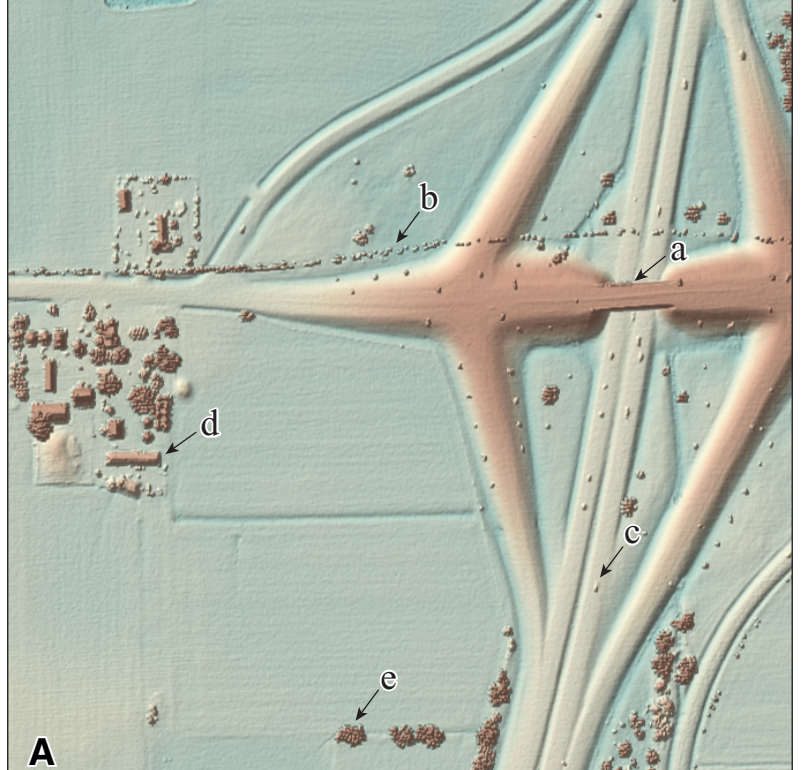
Figure 2 The cross-shaped feature revealed on this digital terrain model (DTM) on Figure 2A (a) is a remnant of an abandoned, underground longwall coal mine referred to as the Diamond Mine (T32N, R09E). A DTM represents only the ground surface and is extracted from airborne LIDAR data using automated filtering methods to produce what is commonly referred to as a "bare-earth" point cloud. Located near Bradwood in Will County, Illinois, the Diamond Mine began operations in February 1883. During the intervening period of 131 years, it has been estimated that approximately 2 feet of ground subsidence has occurred because of the type of hand-mining operation (unpublished manuscript by Robert A. Bauer 2008). This DTM defines not only the belowground structures associated with these mines, such as the supporting pillars or "thelageways" (a), but also the extent of these underground mine operations (b). The 2-foot contours depicted on Figure 2B confirm that at least 2 feet of subsidence has occurred. Contours are shown at 2- and 5-foot intervals. Scale is 1:6,000 (1 in. = 500 ft).
