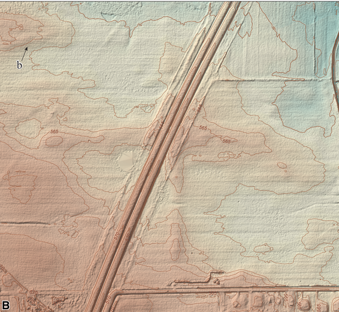
Figure 3 The feature shown is a cloverleaf structure associated with I-55 located at the Will County boundary (T32N, R09E). Figure 3A is a digital surface model (DSM), whereas Figure 3B is a DTM of the same area. In contrast to a DTM, which represents only ground features, a DSM portrays all aboveground features. For example, the roadway overpass (a) shown on the DSM has been removed on the DTM because the elevated roadway is not considered part of the ground surface. Likewise, the patterns of scattered points at (b) on the DSM represent the cables of an aboveground transmission line, which have been removed on the DTM. Vehicles moving along I-55 (c), building structures (d), and trees and other vegetation (e), all of which are visible on the DSM, have been removed on the DTM. Scale is 1:6,000 (1 in. = 500 ft).
