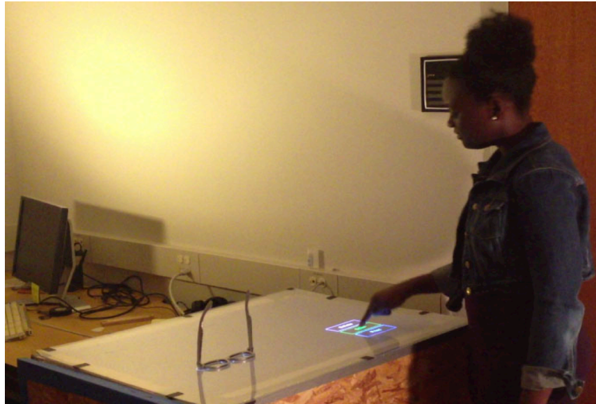
Figure 1. The Easy Make Oven prototype consists of an optical-based interactive tabletop that can track touches and scan physical objects. The Easy Make Oven may be used to create 3D models by manipulating and combining scanned physical objects and sketches. A video demonstration of the Easy Make Oven may be found at http://youtu.be/w3nu07bjl
