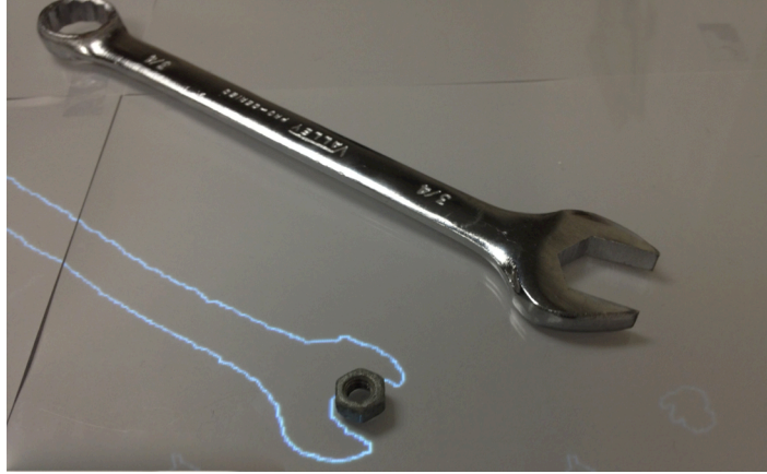
Figure 3. The Easy Make Oven allows users to scan physical objects on a large interactive surface and modify scanned objects using gestures. In this example, the user scans a wrench, and then uses a multi-touch pinch gesture to scale the scanned wrench model to match a physical nut.
