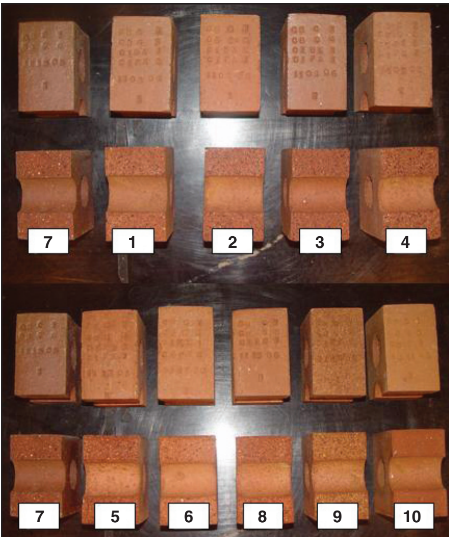
Figure 4 Full-size bricks, sawn in half, after firing at Brick Plant I. Brick 7 is the reference standard commercial formulation brick.
