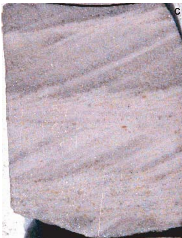
Figure 14 Photograph of core (8.9 cm, or 3.5 inches in diameter) of cross-bedded sandstone facies from (A) Hazen #5 well, 1,251 m (4,105 ft); (B) J. Williams #4 well, 1,279 m (4,197 ft); (C) J. Williams #4 well, 1,228 m (4,030 ft). This medium- to coarse-grained, cross-bedded sandstone is the primary reservoir facies. Cross-beds may be tabular (A) or trough shaped (C). The bases of the cross-beds (B) may have some quartz granules. The thickness of the tabular cross-bed sets ranges from 30 to 100 cm (1 to 3 ft). Trough cross-bed sets typically are only 5 to 15 cm thick (2.5 to 6 in).
