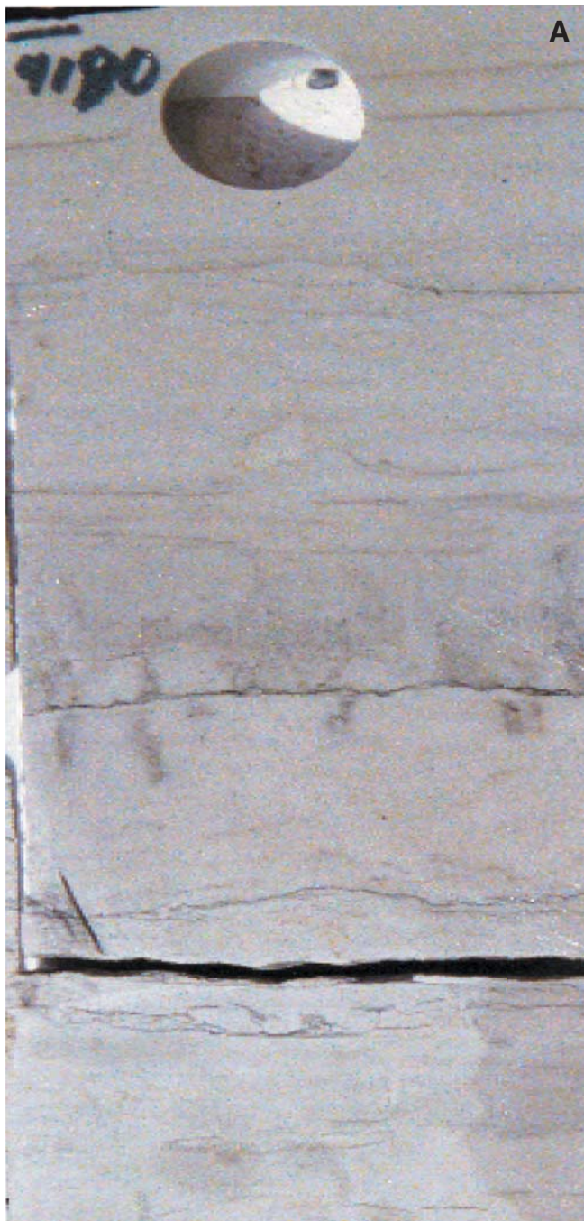
Figure 15 Photograph of core (8.9 cm, or 3.5 inches in diameter) of bioturbated sandstone facies from (A) J. Williams #4 well, 1,274 m (4,180 ft) and (B) Hazen #5 well, 1,221 m (4,005 ft). Vertical Skolithos burrows in medium to coarse sandstone may obliterate most of the original stratification. These burrows are formed from filter feeders that live in a high-energy substrate and intercept food from the moving water that lies above.
