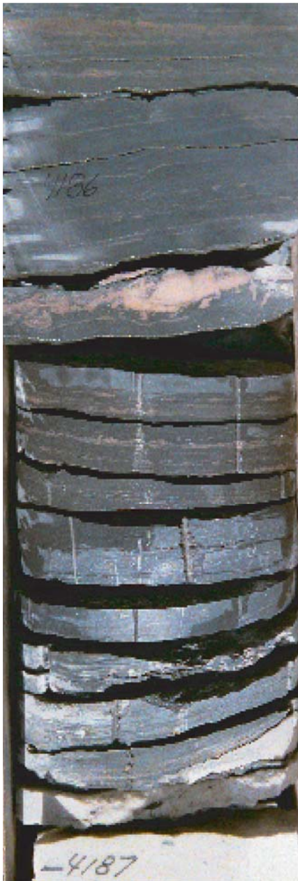
Figure 18 Photograph of core (8.9 cm, or 3.5 inches in diameter) of laminated shale facies from the Hazen #5 well at 1,276 m (4,187 ft). Laminated, dark gray shale with thin laminae of siltstone and local very fine sandstone or siltstone-filled Planolites burrows.
