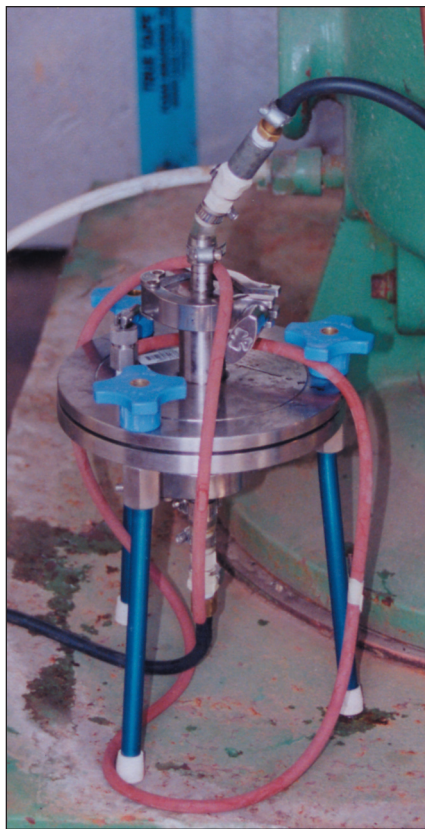
Figure 8 Apparatus used to filter approximately 130 gallons of groundwater through a 0.50- \mu\text{m} Teflon filter. The materials collected on the filter were examined using scanning electron microscopy.
