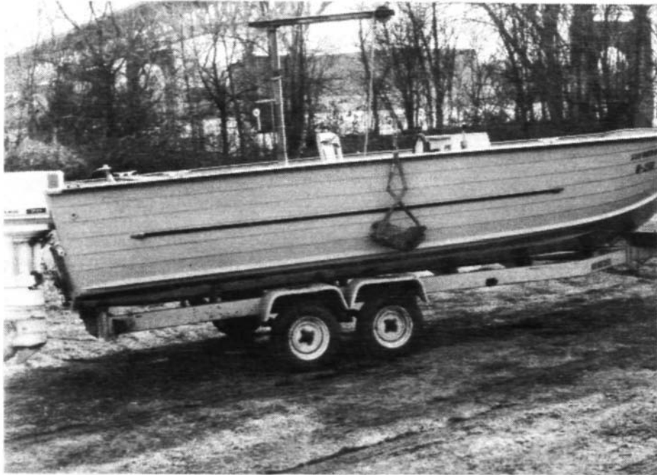
Figure 2. 21-foot semi-vee sampling boat equipped with power winch and Ponar dredge
