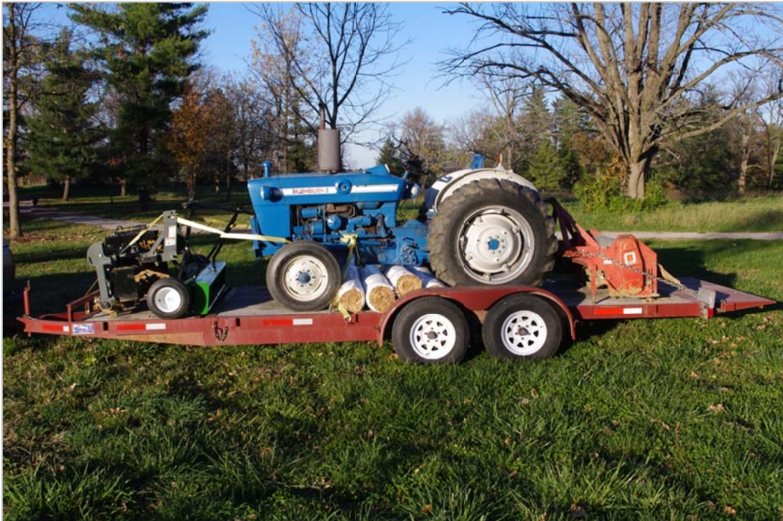
Figure 3. Equipment transport. Power rake, drop seeder, tractor, and tiller loaded for transport to remote planting site.
