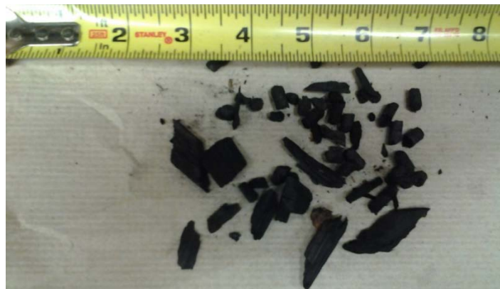
Figure 17. A uniform mixture of pellet char and wood char was found at the bottom of the reactor. Switchgrass pellets were visible in the form of pellet char.
