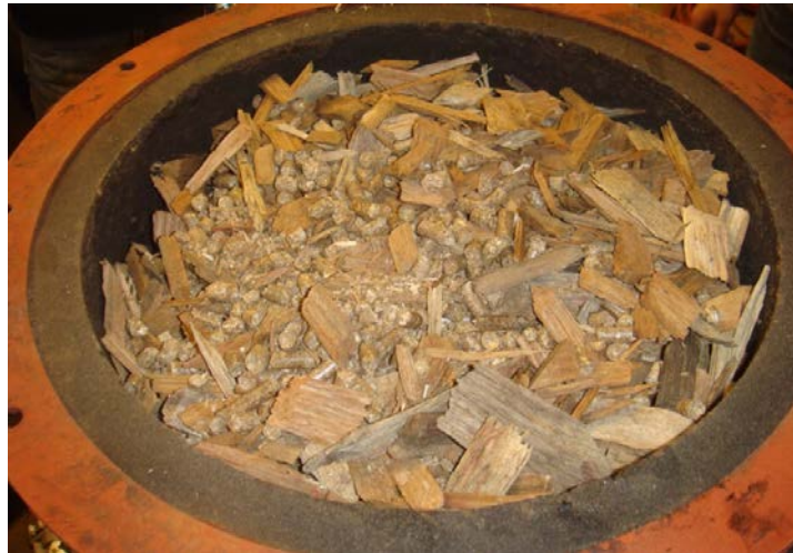
Figure 5. Fuel mix (50% wood chips and 50% switchgrass pellets) in feeding bucket.
