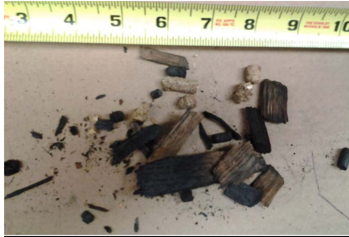
Figure 16. A relatively uniform mix of wood chips and switchgrass pellets was found in the combustion zone.
