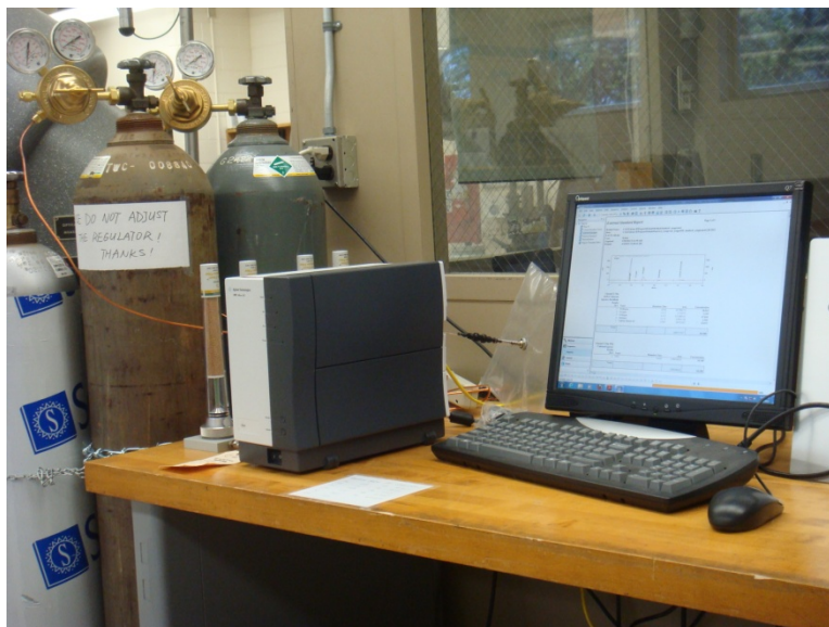
Figure 4. Micro GC used to measure the composition of syngas.
