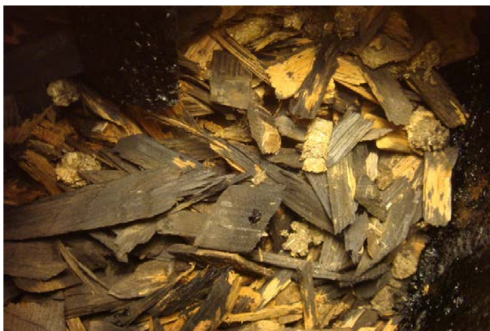
Figure 6. Solid fuel left on top of the gasifier chamber after the gasifier was shut down and cooled.
