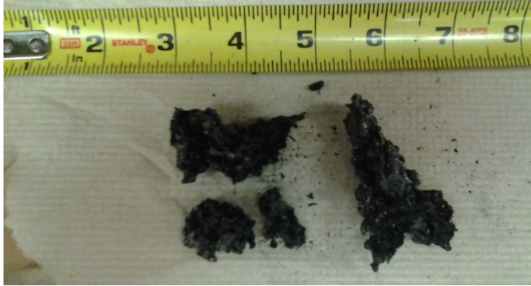
Figure 18. Small clinkers were found in the combustion zone.
