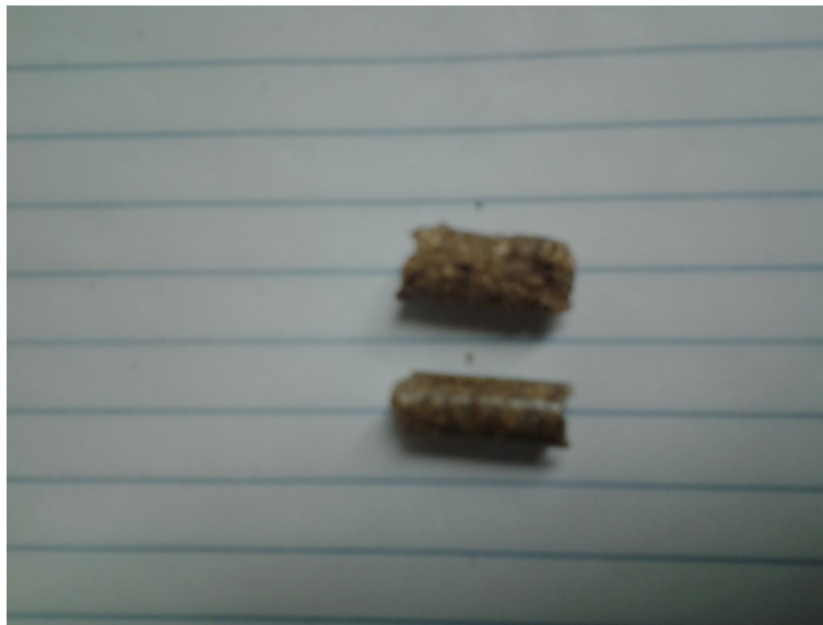
Figure 11. Pellets were deteriorated in feeding bucket after the previous run. Also shown is an unaffected pellet (bottom) for comparison.
