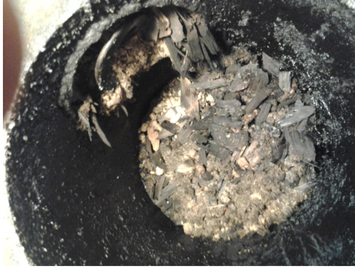
Figure 14. Approximately eight inches from the top opening of the gasifier chamber. Materials were shown to be tarry and somewhat wet.
