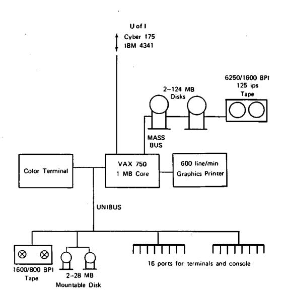
Figure 1. Original proposed DEC VAX 11-750 system.
