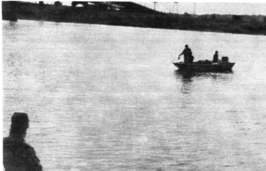
Figure 14. Setting markers using tag line from shore
