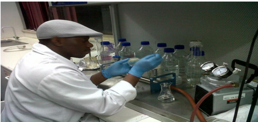
C. Student using membrane filtration set up for bacteriological analysis of effluent samples.
