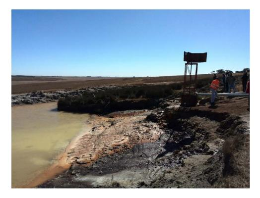
Figure 1.3: AMD decant from closed mine workings in quaternary catchment X11B, near Carolina. The decant had occurred once the mining operation had been seized, and during the plans to rehabilitate the land, the mining company who owned the rights to the land filed for liquidation, which is discussed later on in this work.
