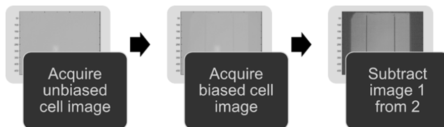
Figure 3-13: IR thermography procedure.
