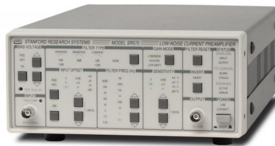
Figure 3-11: SR570 Current Preamplifier [52].
