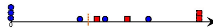
Figure 11. One optimistic prediction of a distance distribution based on distances that have already been calculated in fig. 10. The dashed objects are in the optimistically assumed placements.
