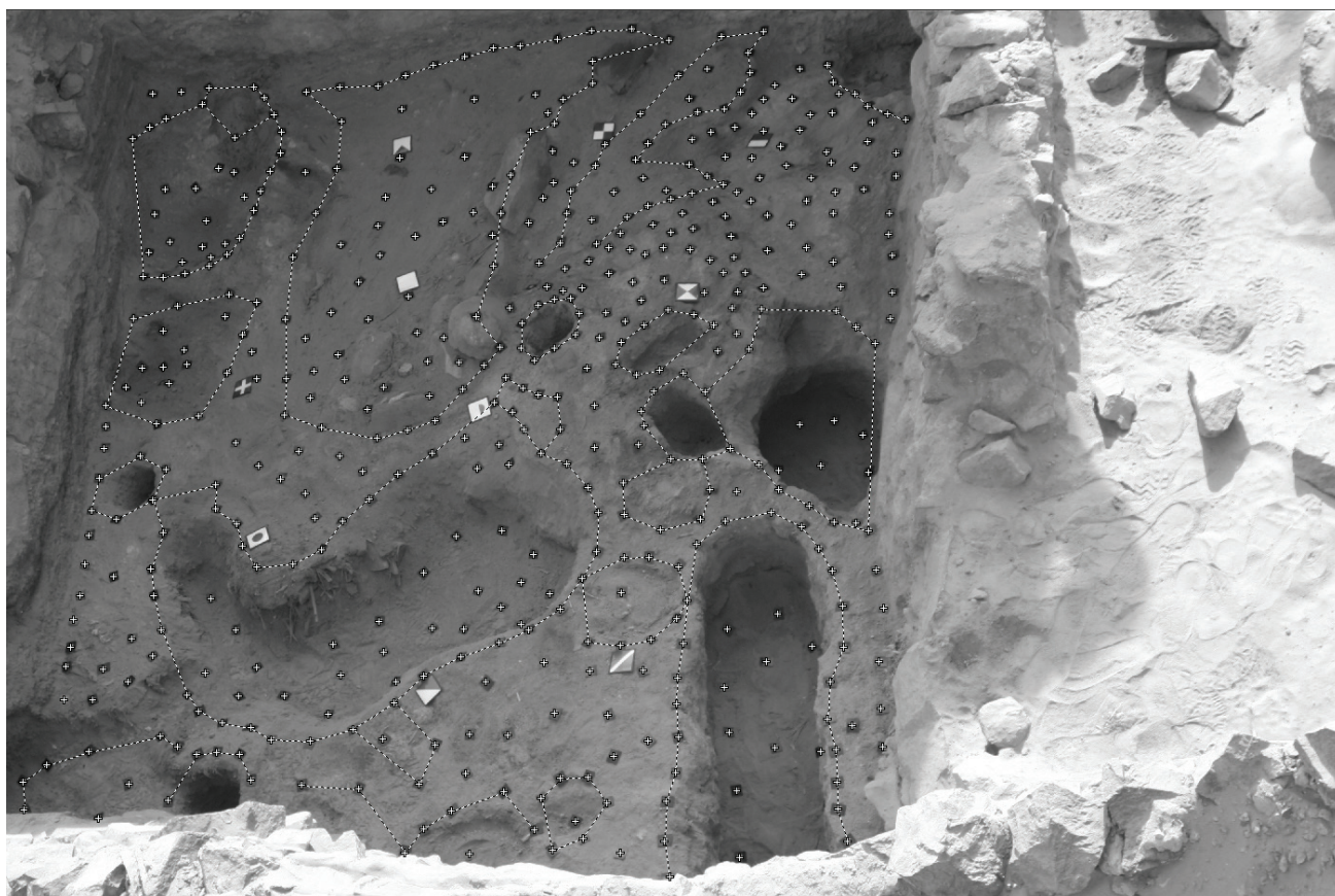
Figure 4. Circular targets placed on a stratigraphic interface at Huayuri. Here, 516 targets have been placed in an area of about 6.5 m 2 . The density, and hence the resolution of the model, could be increased with little extra effort. Feature edges have been outlined with circular targets. The resulting 3D points are easily connected to form 2.5D polygons in a GIS database. A full 3D model may be composed from multiple such polygon slices though a feature that may be difficult to capture otherwise, for example a narrow posthole. Some images in a set may be taken with circular targets removed and only coded targets left on the interface. These images are used to produce orthophotos for publication (cf. Figure 9).
